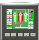
The generator is controlled using the latest in HMI touch screen technology to display the process, pressures, inlet air dewpoint and oxygen levels with continuous monitoring complete with alarms.
